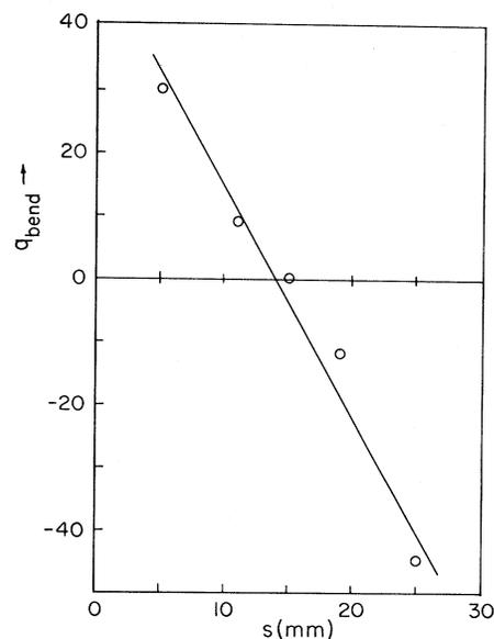
FIG. 3. Rotation fringe rate  $q_{\text{bend}}$ , see Eq. (3), caused by bending of the interferometer base under its own weight, as a function of the position  $s$  of the felt strips from either end of the crystal.
