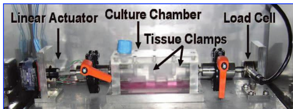
FIG. 1. Cyclic stretching tissue culture (CSTC) system. Color images available online at www.liebertonline.com/ten .
