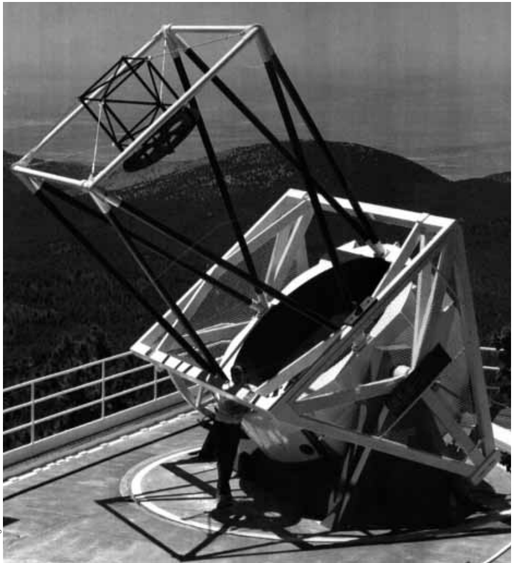
Telescope engineer Charlie Hull poses with the skeleton of the Sloan Digital Sky Survey's 2.5 meter telescope shortly after it was installed.
