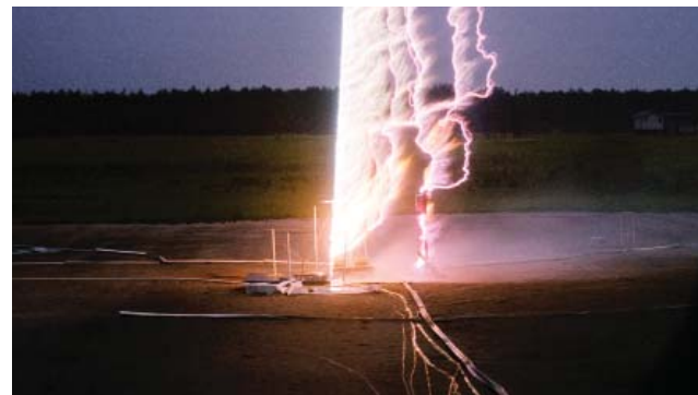
Lightning strikes. A rocket-triggered lightning flash striking on or near a short rod at the ICLRT.
