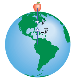
Fig. 14-3: The apple pulls up on Earth just as hard as Earth pulls down on the apple.
