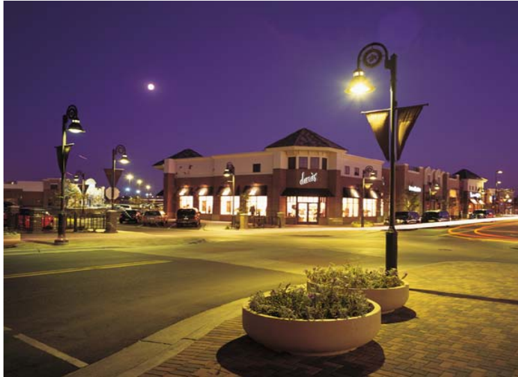
Shopping district “architectural” street lighting meeting aesthetic and cutoff requirements
