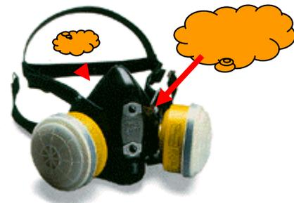
The **Assigned Protection Factor (APF)** of a respirator reflects the level of protection that a properly functioning respirator would be expected to provide to a population of properly fitted and trained users. For example, an APF of 10 for a respirator means that a user could expect to inhale no more than one tenth of the airborne contaminant present.
