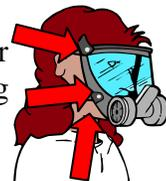
**Fit Factor** is a quantitative measure of how well a particular respirator fits an individual. It is defined as the ratio of the concentration of a contaminant in the environment to the concentration inside the mask. Fit Factors are obtained from **Quantitative Fit Testing**.
