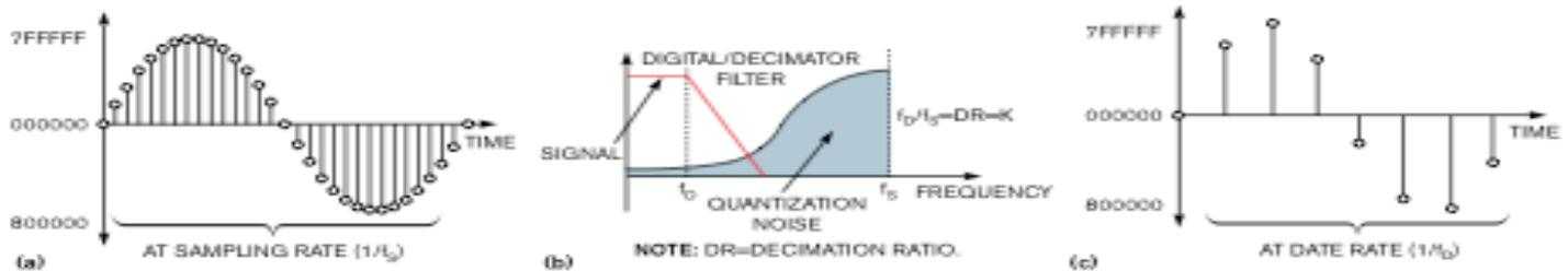
**Figure 1** The digital-filter output function produces a high-resolution result (a), while rejecting high-frequency noise (b). The decimator function slows the output data rate (c).
