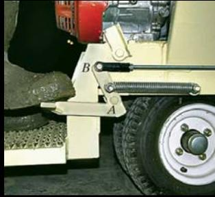
**Given:** The operator applies a vertical force to the pedal so that the spring is stretched 1.5 in. and the force in the short link at  $B$  is 20 lb.
