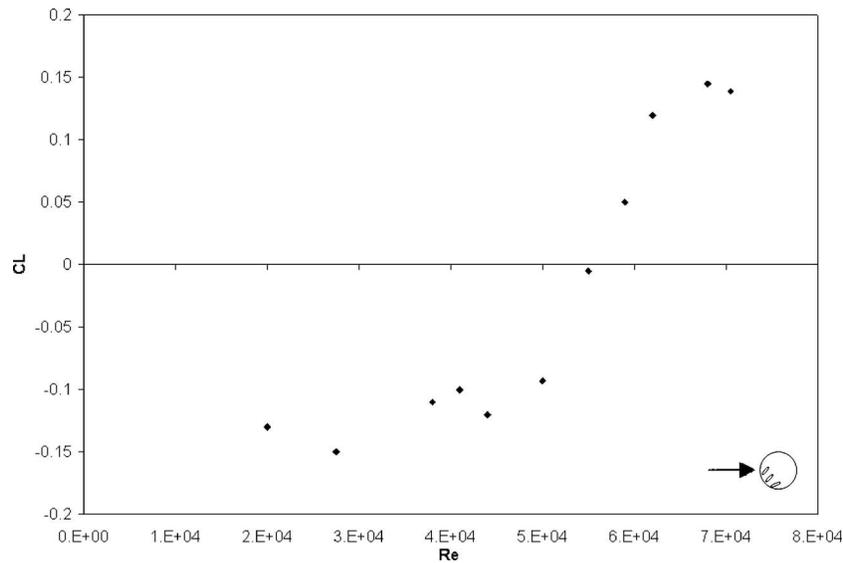
Fig. 9. The change of sign of the lift coefficient versus Reynolds number for  $\beta=345^\circ$ .
