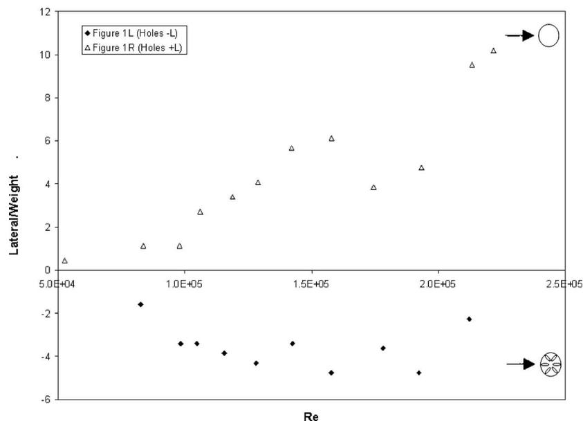
Fig. 10. The ratio of lateral force to Wiffle ball weight as a function of  $Re$  for holes on the side of ball. Positive lateral force is into the page in ball schematics.
