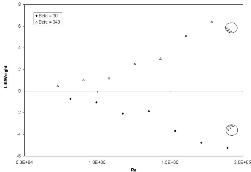
Fig. 7. Lift-to-weight ratio for a Wiffle ball as function of  $Re$  for holes oriented in the northern ( $\beta > 0^\circ$ ) and southern ( $\beta < 0^\circ$ ) hemispheres.
