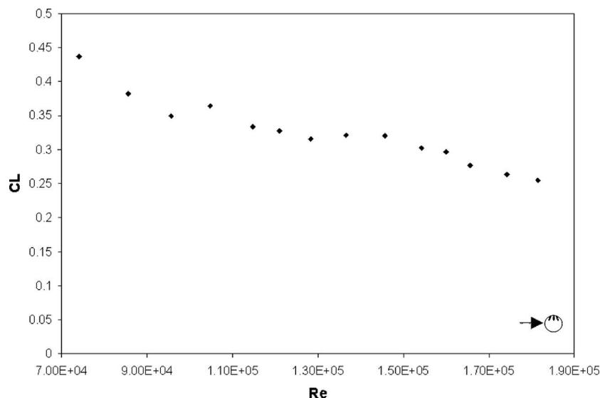
Fig. 8. The lift coefficient as a function of the Reynolds number for a ball with  $\beta = 90^\circ$ .
