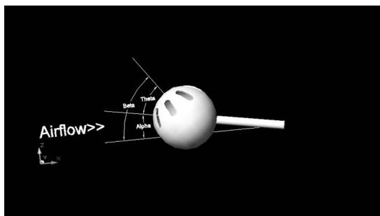
Fig. 2. Orientation of Wiffle ball for wind tunnel experiments.
