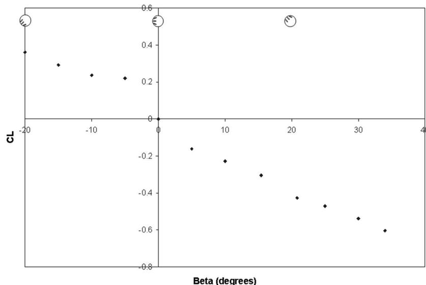
Fig. 6. Variation of lift coefficient with ball orientation characterized by the angle  $\beta$  at  $Re=1 \times 10^5$ .
