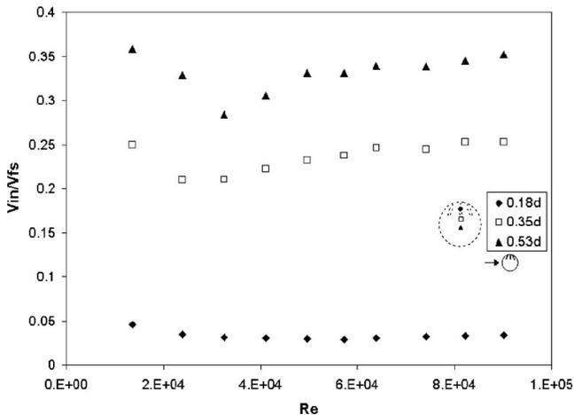
Fig. 12. The ratio of the velocity inside the Wiffle ball to the free stream velocity,  $V_{in}/V_{fs}$ , at three positions inside the Wiffle ball.  $\beta=90^\circ$ .
