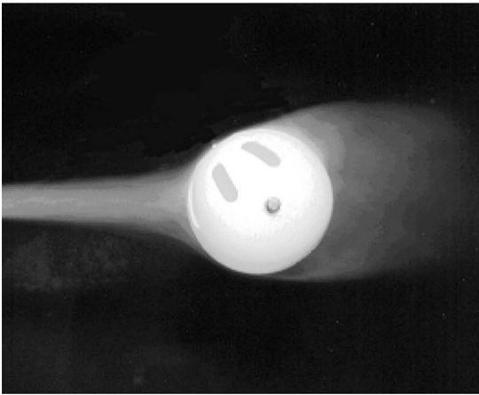
Fig. 5. (a) Symmetric layout of Wiffle ball holes. (b) Upward deflection of Wiffle ball wake due to asymmetric position of the holes. Fog visualization images taken at  $Re=4 \times 10^4$ . The observations were determined to be independent of string balance position.
