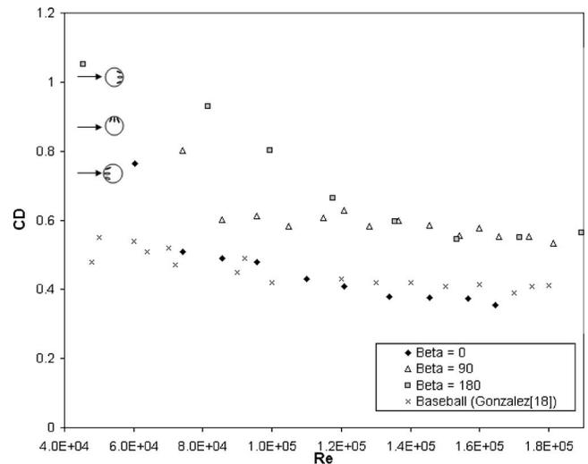
Fig. 3. Wiffle ball drag coefficient as function of the Reynolds number for various orientations.
