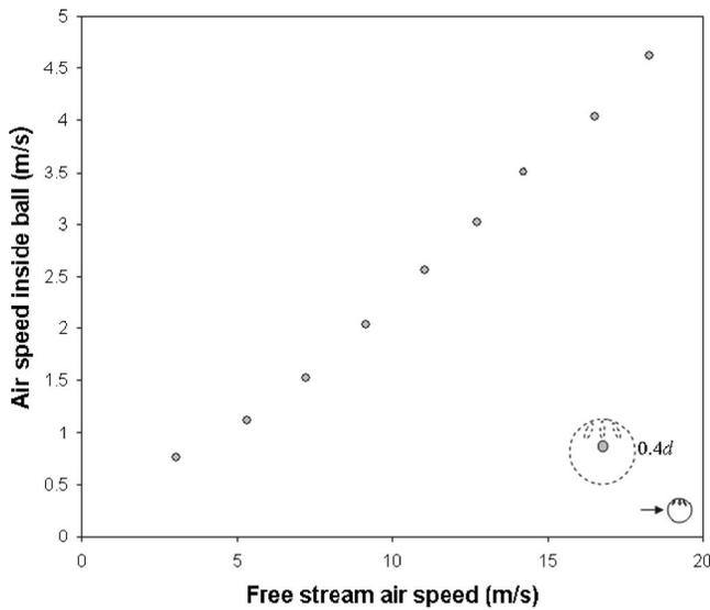
Fig. 11. Velocity  $0.4d$  inside the Wiffle ball versus the free stream (outside) velocity.  $\beta=90^\circ$ .
