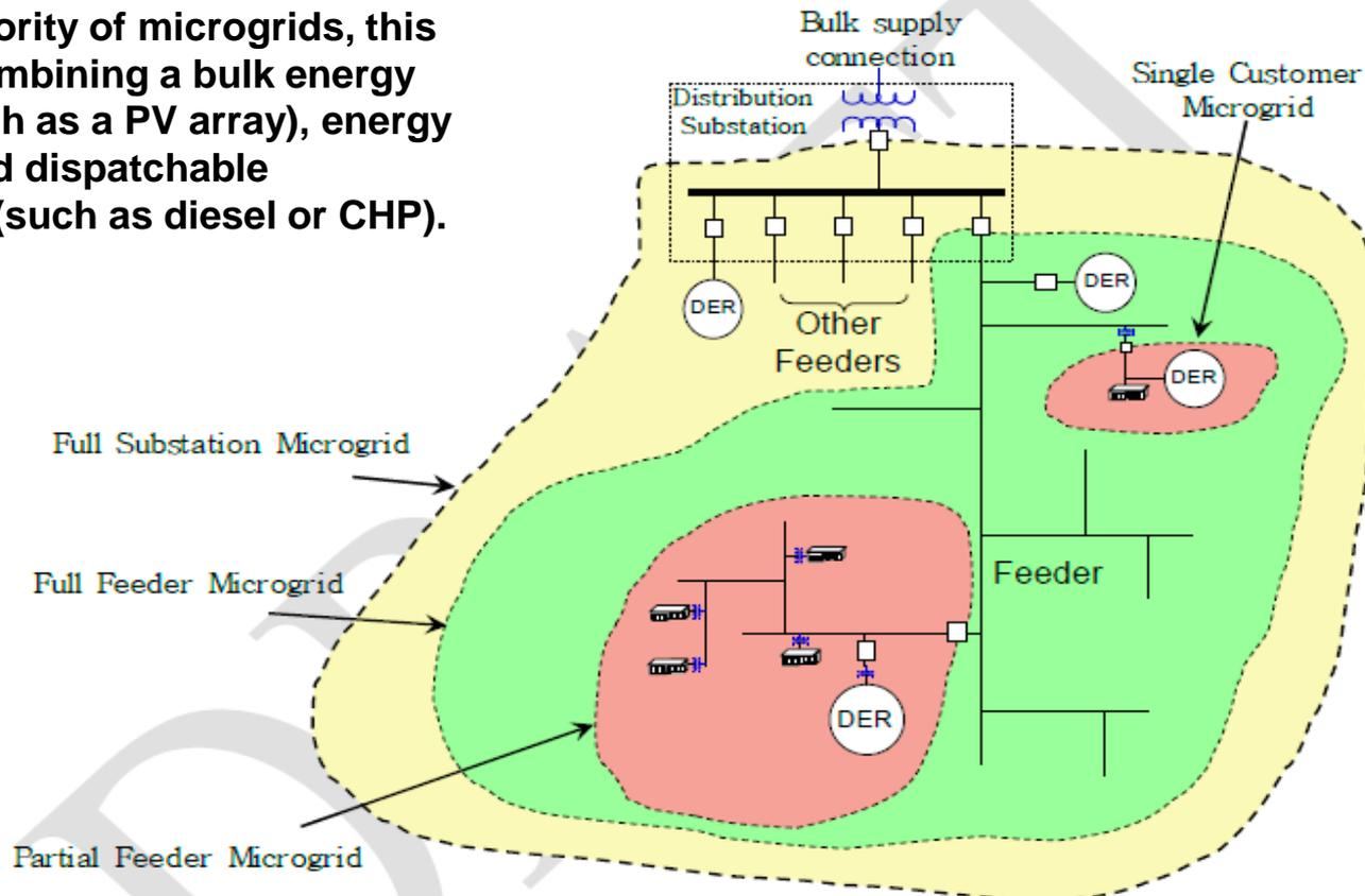
Figure 4: Examples of Microgrid Architecture on a Radial Distribution System – From Single Customer up to the Entire Substation
